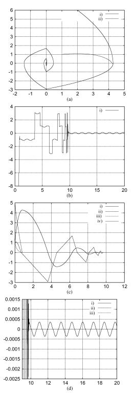
Fig. 6. Simulation of (60) with  $\varphi(t) = \phi \sin(\omega t)$ ,  $\phi = 0.1$ ,  $\omega = 5$ . (a) Phase portrait. i) State  $x_k$  versus  $y_k$  ii) observer  $\hat{x}_k$  versus  $\hat{y}_k$ ; (b) control versus time i)  $u_k$ ; (c) state and error versus time i)  $\hat{x}_k$  ii)  $\hat{y}_k$  iii)  $e_{1,k}$  iv)  $e_{2,k}$ . (d) Sliding variable versus time. i)  $\operatorname{sgn}(\hat{y}_k)$  ii)  $\operatorname{sgn}(e_{1,k})$  iii)  $\operatorname{sgn}(\tilde{x}_k)$ .
