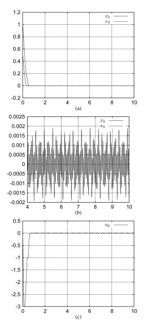
Fig. 2. Simulation of the system (10) with  $\varphi(t)=\phi\sin\omega t$ ,  $\phi=0.1$ ,  $\omega=100$ . (a) State versus time (fine sampling). (b) State versus time (fine sampling, zoom). (c) Control input u(t).
