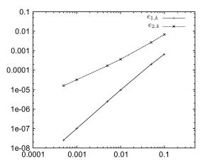
Fig. 7. Double logarithmic plot of the attenuation of the disturbance with respect to the sampling time.
