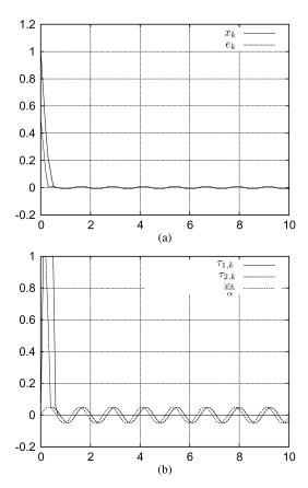
Fig. 1. Simulation of the system (10),  $\phi=0.1, \omega=5$ . (a) State  $x_k$  and error  $e_k$  versus time; (b) multiplier  $\tau_{1,k+1}, \tau_{2,k+1}$  and perturbation  $\varphi_k/\alpha$  versus time.
