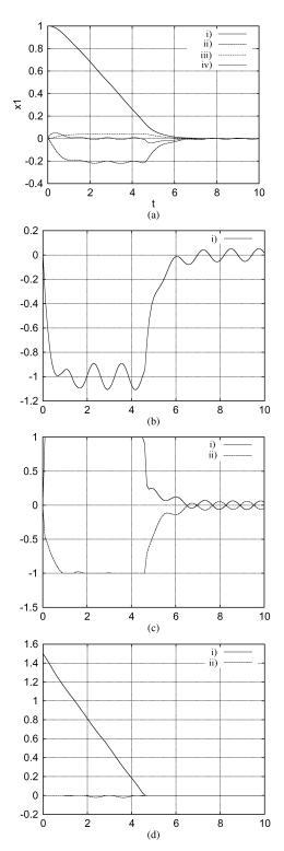
Fig. 5. Simulation of (44) with  $\varphi(t)=\phi\sin(\omega t)$ ,  $\phi=0.1$ ,  $\omega=5$ . (a) State versus time (fine sampling): i)  $x_k$ , ii)  $\dot{x}_k$ , iii)  $e_k$ , iv)  $\dot{e}_k$ . (b) Control versus time i)  $u_k$ . (c) Multiplier versus time: i)  $\tau_{1,k}$ , ii)  $\tau_{2,k}$ . (d) Sliding variable i)  $s_{x,k}$  ii)  $s_{x,k}$  ii)  $s_{x,k}$  ii)
