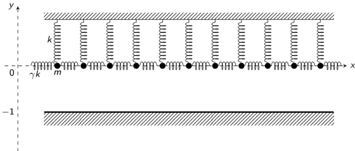
Figure : A chain of linearly coupled impact oscillators
